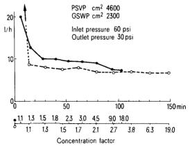
Filtrate flow levels during the concentration of *B. pertussis* by tangential filtration using PSVP anisotropic (•) and GSWP microporous (O) membranes. Starting volumes: 18 l for PSVP membranes and 19 l for GSWP membranes. The high initial flow (not estimated) and the rapid passage to a steady flow rate in the case of the microporous membranes, are indicated by the arrow and the dotted line
